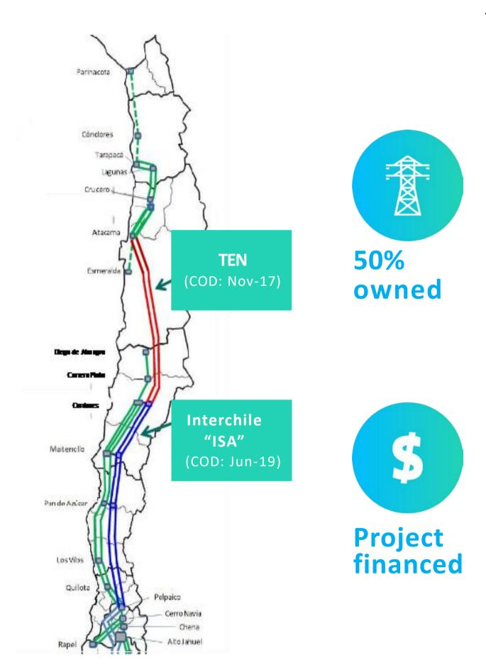
Double circuit, 500 kV, alternate current (HVAC), 1,500 MW, 600-km long transmission line
