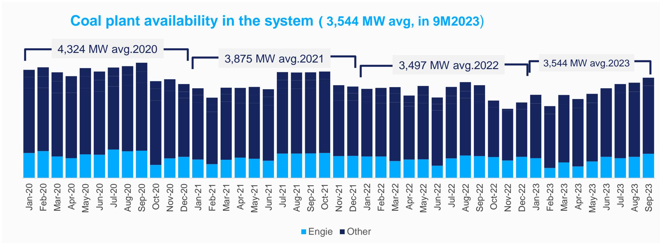
The avg unavailability for 2023 to sept (YTD) calculated as the difference between the maximum capacity of all the coal units in the system vs the average available capacity (YTD), was ~ -813 MW-month
